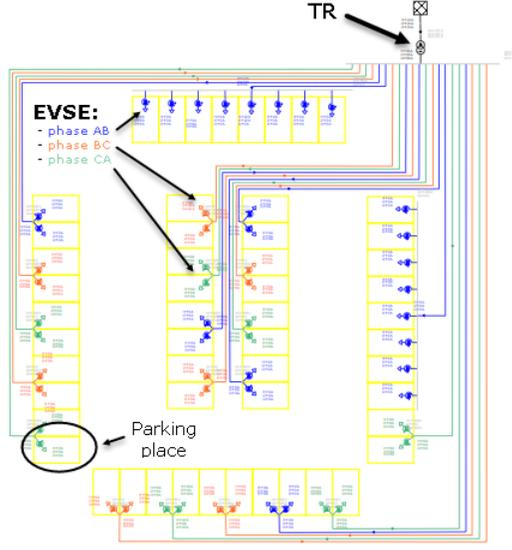
**Figure 1: Electrical installation for an EV parking lot with charging stations. TR denotes the installation transformer and EVSE the different charging pods.**
